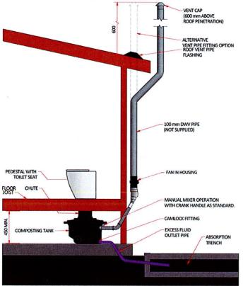
operate aerobically with vented air circulation and a small land application system to absorb urine.
