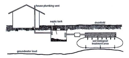
The most common on-site wastewater management systems are septic tank (ST) installations (see above diagram) and aerated wastewater treatment system (AWTS) installations:
