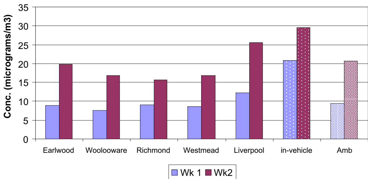
Figure 4. Comparative PM 2.5 concentration levels: AQMN site, in-vehicle and actual time ambient exposure estimate (Amb) for car commuters
