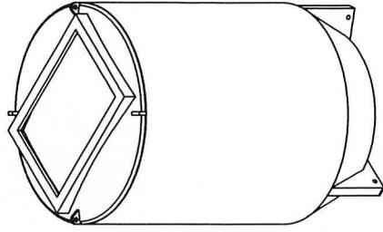
1400 diameter SPE Collection Wells are available with either 600mm circular opening or 900mm x 600mm rectangular opening.
