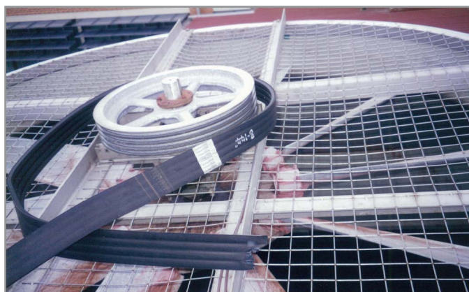
Figure 5.4-1: Broken fanbelt where the motor functions but the fan does not
