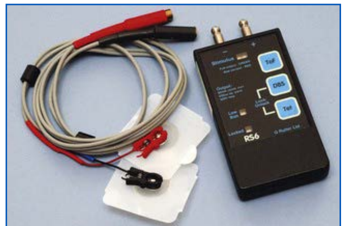
Figure 3-9. Neuromuscular ('train of four') monitor: usually applied over the ulnar nerve or facial nerve.
