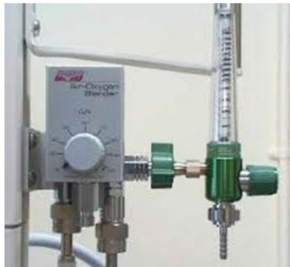
Example of external Air/Oxygen blender
