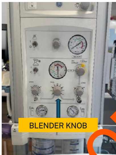
Figure 1. Image of a GE Healthcare resuscitaire beds (infant warmer) showing the potentially impacted oxygen blender knob
