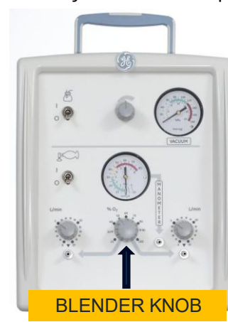
Figure 2. Image of a GE Healthcare Giraffe Stand-alone Infant Resuscitation System showing the potentially impacted oxygen blender knob
