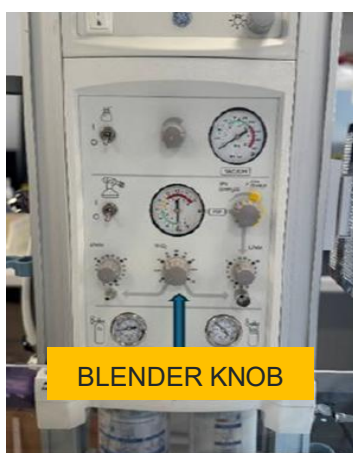
Figure 1. Image of a GE Healthcare Giraffe and Panda warmers with Integrated Resuscitation System (iRes) showing the potentially impacted oxygen blender knob
