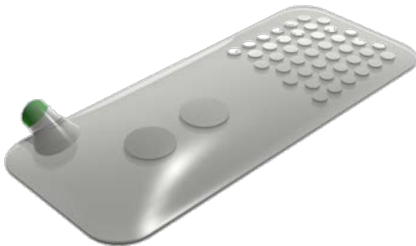
High-density Pt electrodes on a medical grade silicone carrier
